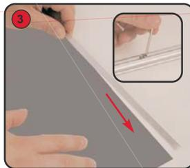
Adhere the flat bar to the back of the graphic. Slide the flat bar and graphic into the top rail. Tighten the screws to secure the top rail. Close the rail end cap.
